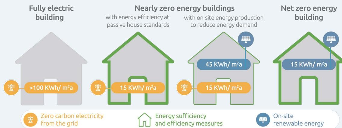
Figure 4: Different options for decarbonising buildings include electrification of equipment, improvements to the building envelope to reduce energy demand, and the installation of on-site renewable energy. Each of the buildings shown here combine these elements in different ways but all are zero carbon when the grid is zero carbon.
