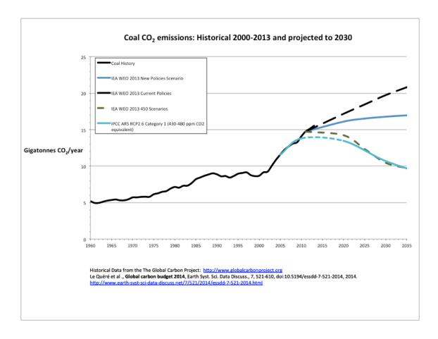
Figure 1 Historical  $CO_2$  emissions from coal compared to estimated future emissions based on IEA World Energy Outlook 2013 scenarios. The IPCC RCP 2.6 scenario limits warming below 2°C with likely probability. Shown here is the median of model results for estimated  $CO_2$  emissions from coal.
